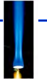
Sandia flame D Jet diam. = 7.2 mm Pilot dia = 18.2 mm Jet U = 50 m/s Coflow U = 0.9 m/s
