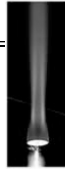
Sandia flame D Jet diam. = 7.2 mm Pilot dia = 18.2 mm Jet U = 50 m/s Coflow U = 0.9 m/s
