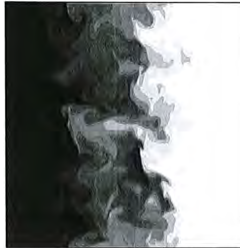
Fig. 1 Slice through the a turbulent region. Nonpremixed turbulent combustion occurs at the interface of the fuel (black) and oxidant (white).
