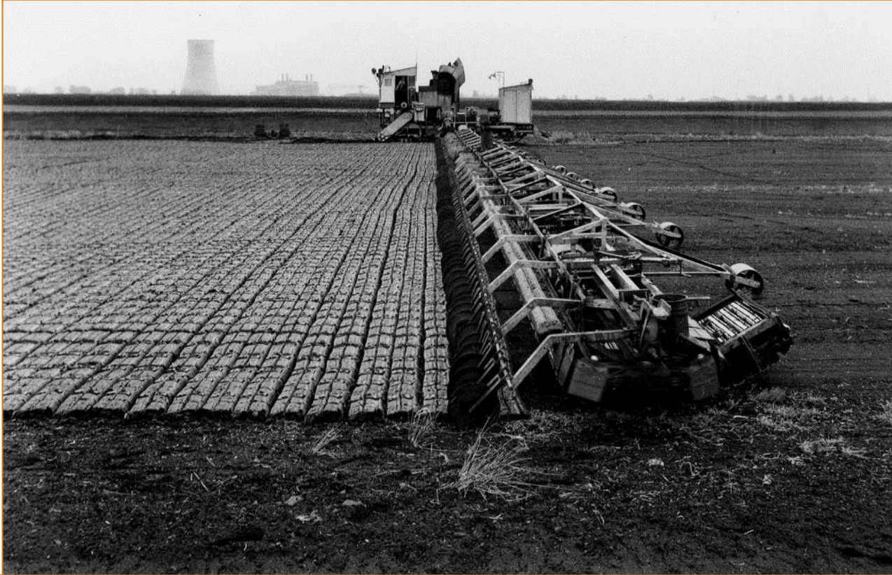
An electrically-powered Bagger, which cut and spread the turf
