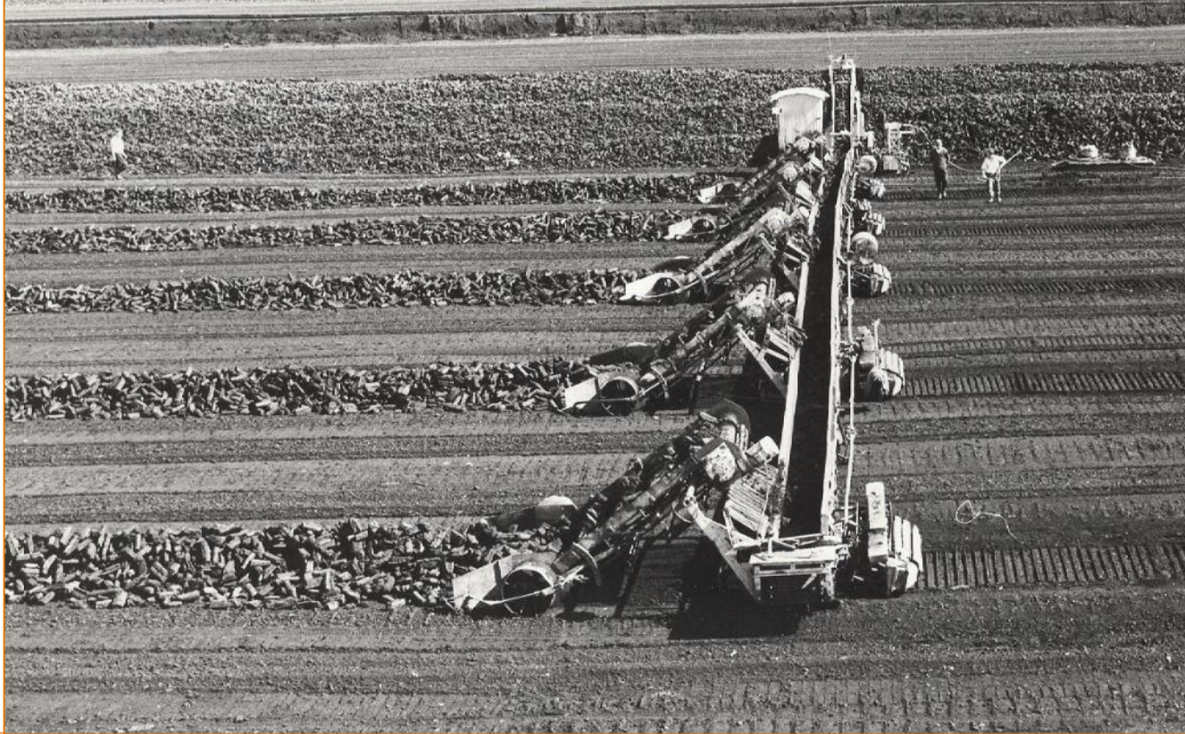
Bord na Móna - fully automated collection of sod turf
