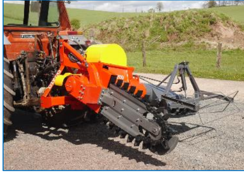
Chain excavator machine
